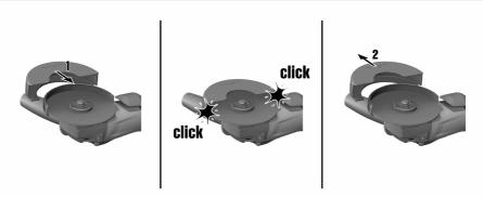
Position the compact guard so that the on/off switch remains easily accessible and operable at all times.
