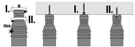
Turn the adjusting ring to the desired torque setting.
