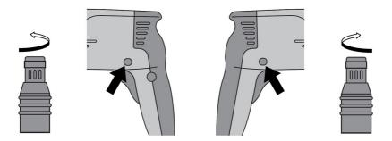
• Set the forward/reverse switch to the desired direction of rotation.
