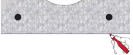
3. Marking pre-stressed steel position
