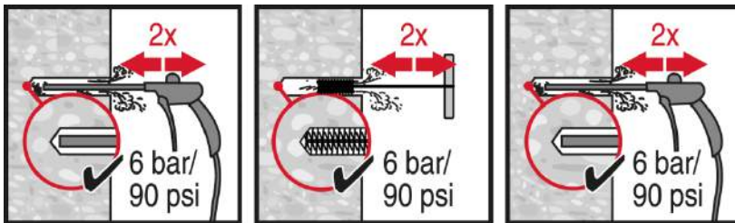
Compressed air cleaning (CAC)
