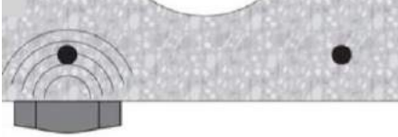
1. Positioning pre-stressed steel
